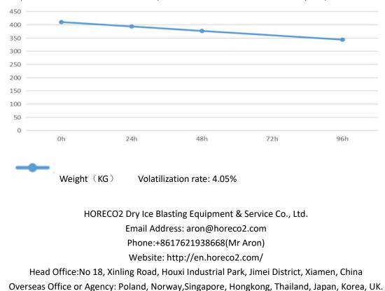
Temperature test chart: Ambient temperature: 26-33°C Load: 3mm dry ice pellets
